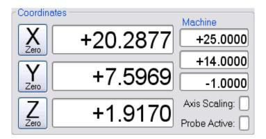
Current X, Y, and Z coordinates are displayed in large DRO's. Buttons to the left of the DRO's will reset their values to zero. When an axis is Referenced (Homed), it's corresponding zero button will have a green border.
